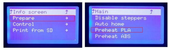
After the extruder temp. reach 180 °C. Operate as below. Pic.54
